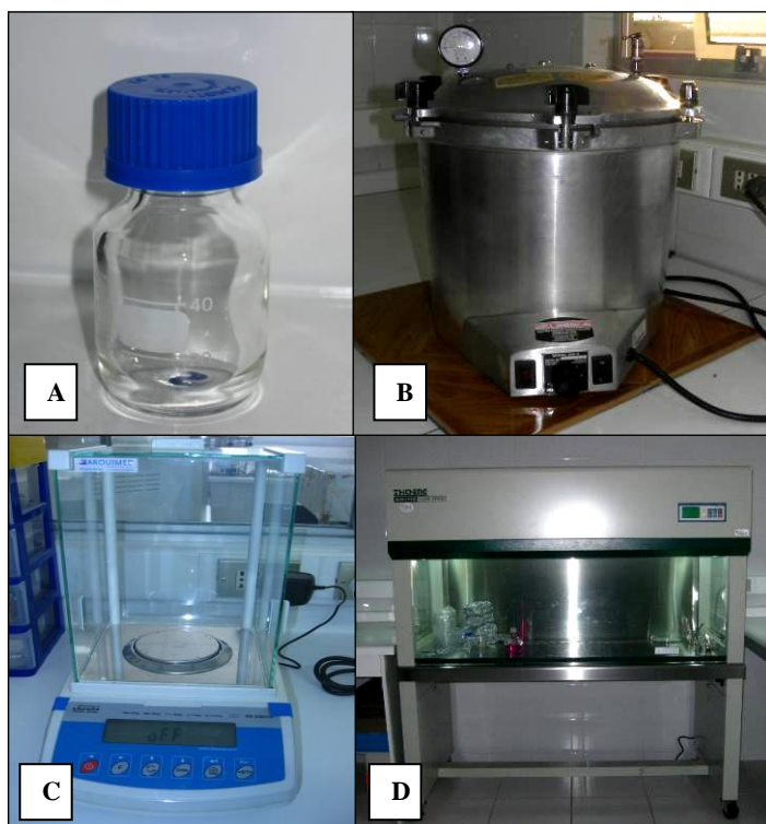
Figura 6. A) Frasco Schott de 40 mL; B) Autoclave All American modelo 25x Electric Pressure Steam Sterilizer; C) Balanza analítica Rodwag modelo AS 220/C/2; D) Campana de flujo laminar vertical Zhicheng modelo ZHJH-C1112C Clean bench.
